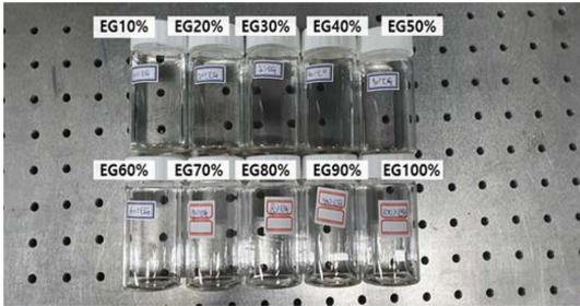
Fig. 5 Prepared samples of ethylene glycol(EG)-water(W) binary mixture
