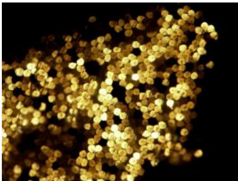
Figure 7. Microscope image of the spun yarn(Dark area is SiC fiber, Bright area is p-Aramid fiber).
