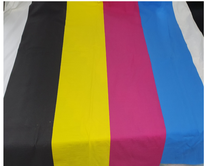
Figure 6. HTPE plain fabric dyed with direct DTP process.
