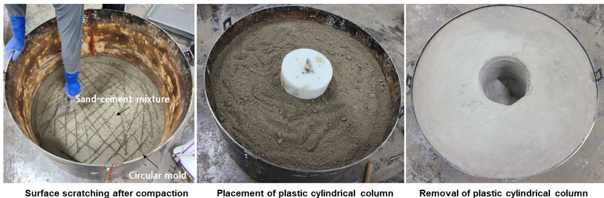
Fig. 6. Preparation of model weathered rock
