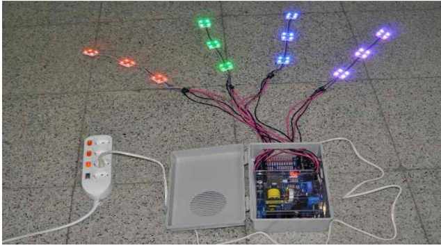
Fig. 8. Operating photograph of four-channel LED lighting control system.
