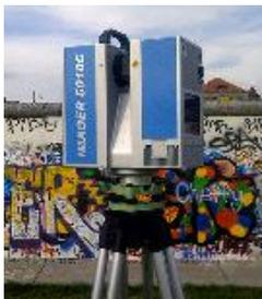
FIGURE 1. 3D Laser scanner (Model: Z+F IMAGER 5010C)
