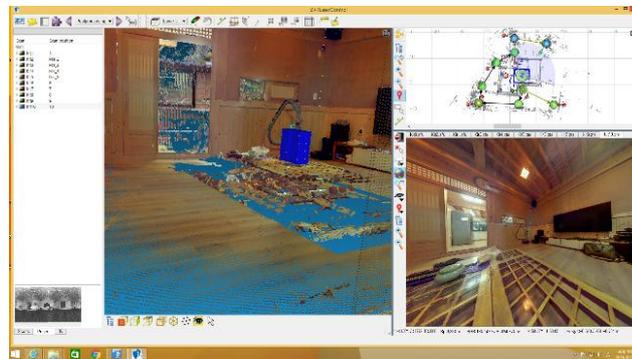
FIGURE 10. 3D model of house inside created based on the scan data of St.10
