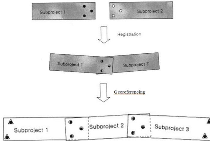
FIGURE 2. The diagram of registration and georeferencing of continuous scan data
