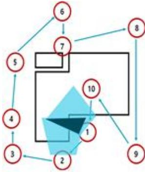
FIGURE 6. Ten laser scanning stations
