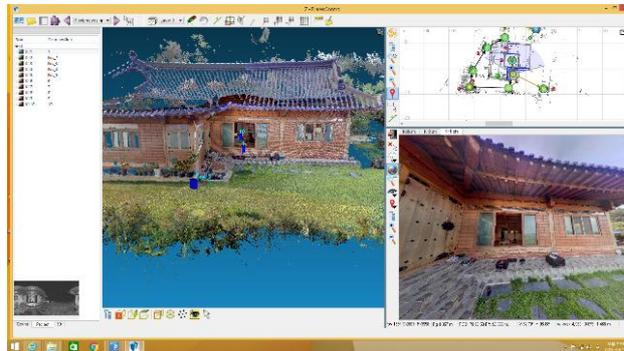
FIGURE 7. 3D model created based on the scan data of St.1
