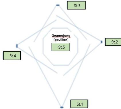
FIGURE 4. Five stations of terrestrial laser scanner
