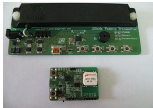
**Fig. 2** 125KHz Wake-up Module[11]
