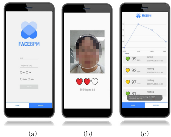
Fig. 4. Screen shots of the mobile application: (a) requiring user information, (b) capturing face images, and (c) displaying heart rate prediction result.
