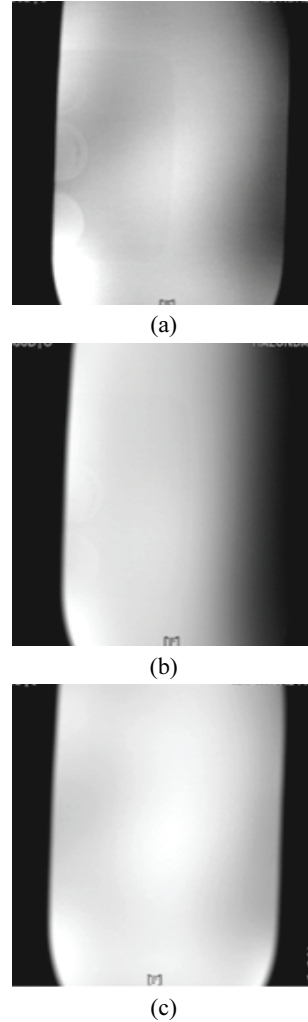
Fig. 5. Phantom images fixed FOV 170mm × 170mm (a) Mesh not used (b) Mesh is placed in the center (c) Mesh is wrapped.
