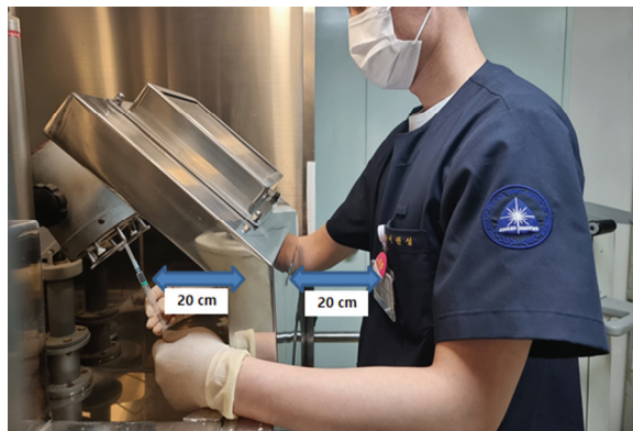
Fig. 1. Distance between source and shield and subject during manual distribution work.
