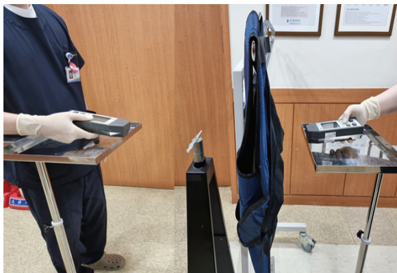
Fig. 4. Spatial dose rate measurements by radiation shield.
