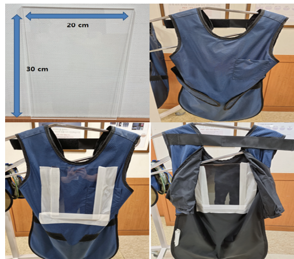
Fig. 3. Radiation Shields established in consideration of the possibility of Bremsstrahlung.
