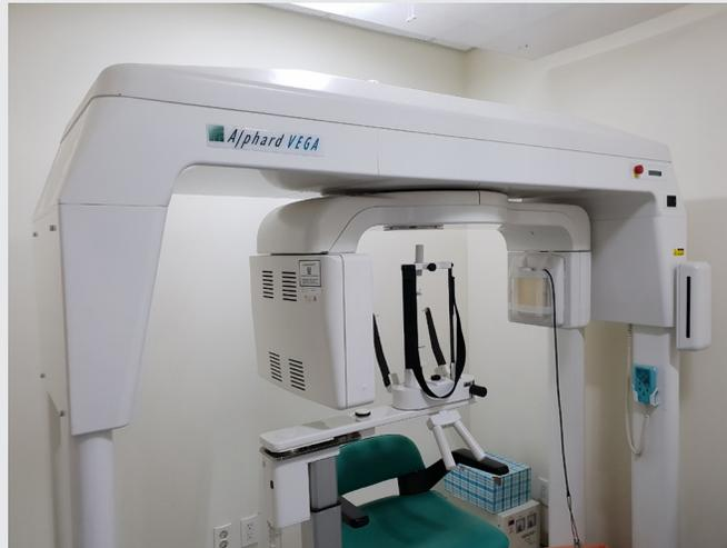
Fig. 2. Ionization chamber of DAP meter is located at the tube side of CBCT scanner for the DAP measurement.
