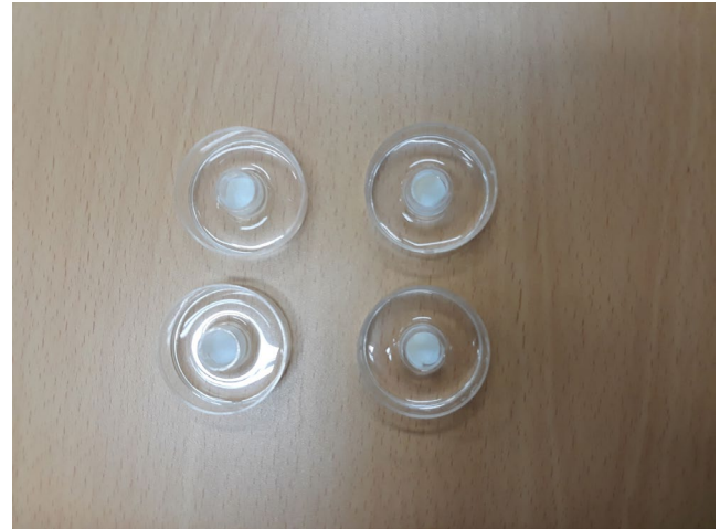
FIGURE 7 Four Petri dishes with inserts for 3D cell culture
