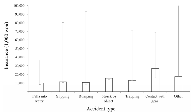
Fig. 4. The hazard assessment using payment of insurance proceeds by accident occurrence patten over the last 3 years in coastal purse seiners.
