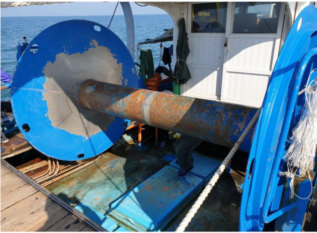
Fig. 3. Differences in net hauler systems between hauling drum in Chungnam sea area (a) and halving roller in Gyeongnam sea area (b).
