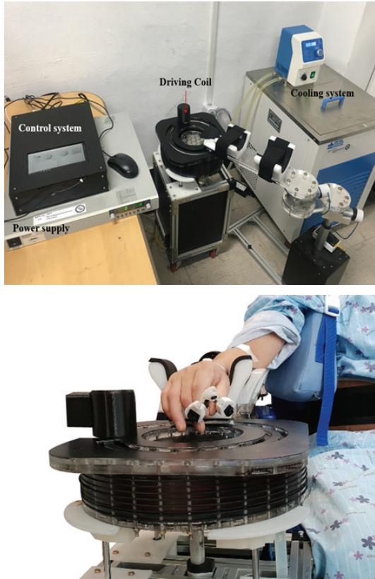
Fig. 1. Hand rehabilitation device using a magnetic force. (A) Electromagnetic fields generated in the coil and permanent magnets worn on the patient's fingers generate an attractive or repulsive force. (B) Rehabilitation therapy was performed by assisting the movement of the paralyzed finger using these magnetic forces.
