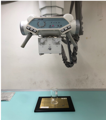
(a) The distance between the x-ray device and the instrument was set to 100 cm
