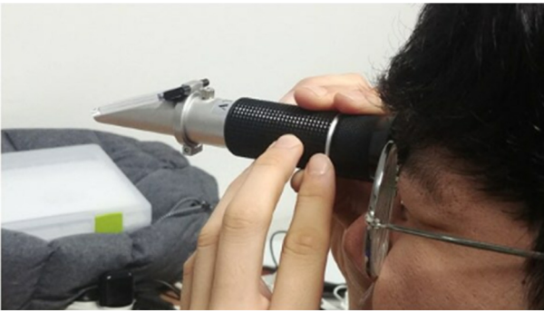
Fig. 5. Destructive brix measurement for obtaining Target
