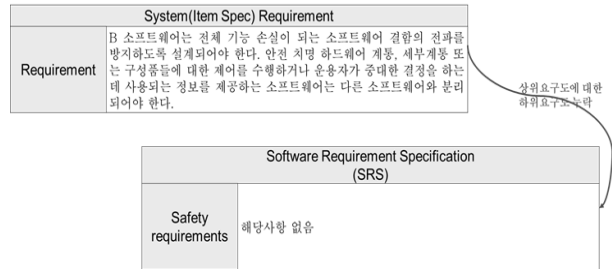
Fig. 5 Missing Lower Requirement for Higher Requirement
