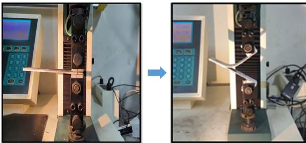
Fig. 2. Photograph of DCB specimen by mode I test.
