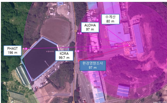
Fig. 11. Comparison of the extent of damage from leak sources.
