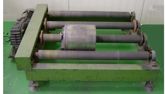
Fig. 2 Ball mill equipment for material mixing
