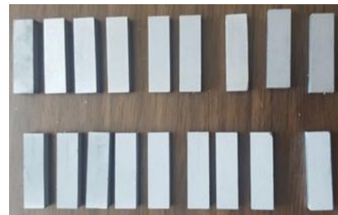
Fig. 5 Cemented carbide specimens after sintering
