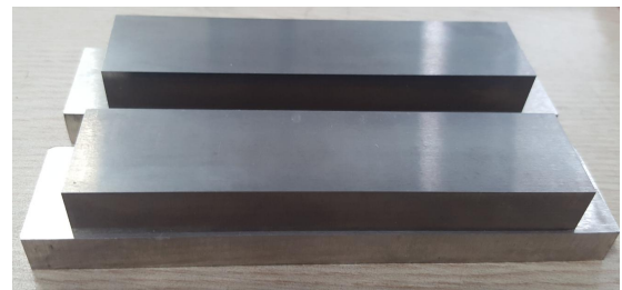
Fig. 7 Cemented carbide tip and stainless steel body after polishing
