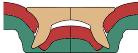
Fig. 5 (a) Simulation results according to the initial thickness of the lower sheet: 1.2t
