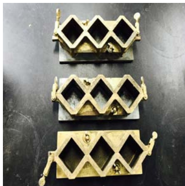
Fig. 2. Steel form and strength meter(Hydraulic Servo Universal Testing Machine 100KN) in using experiment.
