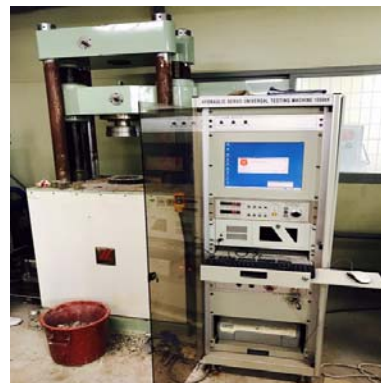
Fig. 2. Steel form and strength meter(Hydraulic Servo Universal Testing Machine 100KN) in using experiment.
