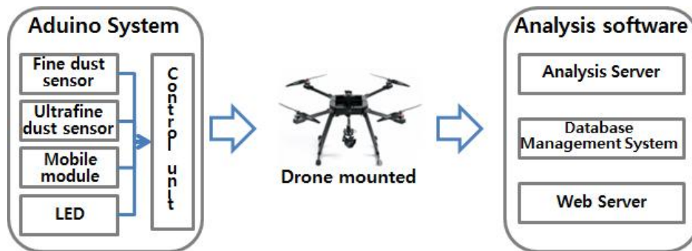
Figure 3. Drone configuration diagram for fine dust measurement
