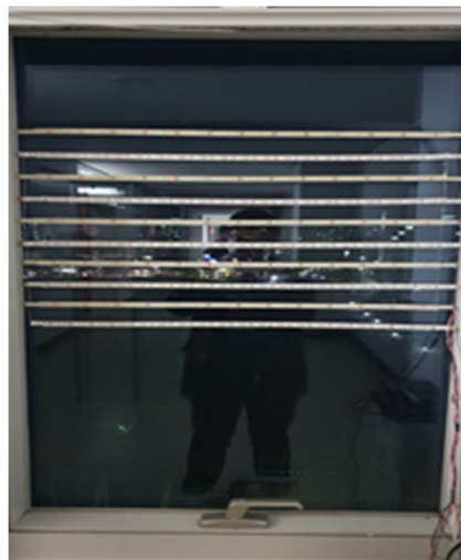
Figure 3. LED pattern attached window signage
