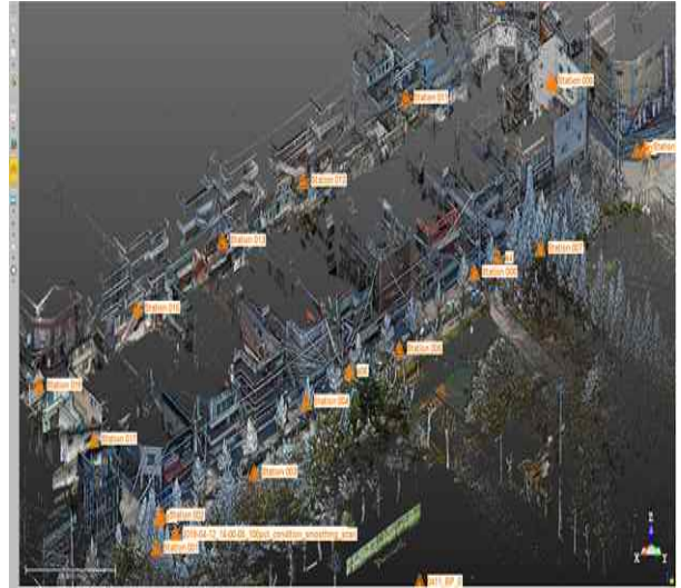
Fig. 7. Data Acquired using a Static 3D Scanner
