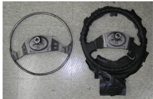
Fig. 1. Application example of RIM process: automobile steering wheel
