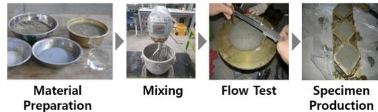
Fig. 2. Manufacturing process of concrete specimens
