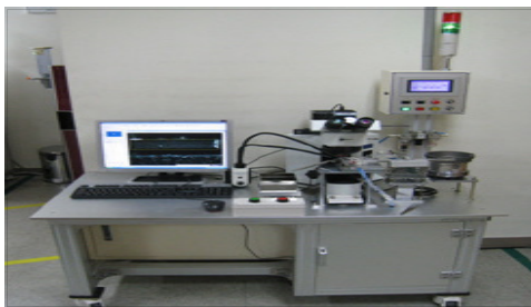
Fig. 8. Molybdenum pin vision inspection device manufactured after design
