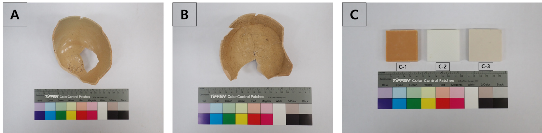
Fig. 1. Research materials(A : glazed pottery, B : unglazed pottery, C : property experiment sample (C-1 : L-30 resin, ABS resin, ceramic resin))
