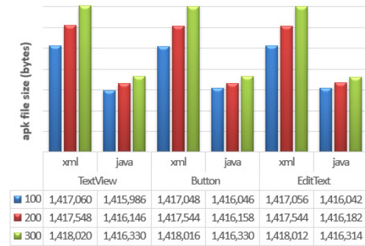
Fig. 11. The apk file size comparison between xml and Java
