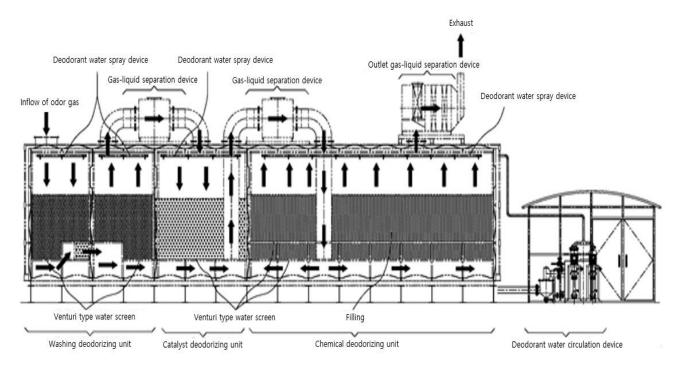
Figure 1: Step-type liquid catalyst chemical liquid deodorizer configuration device
