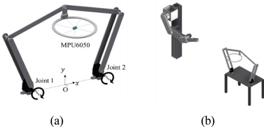
[Fig. 4] (a) Parallel goal post parallel robot, (b) Overall System
