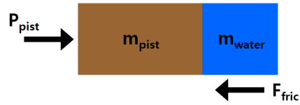
Fig. 5. Force acting on the piston and water column
