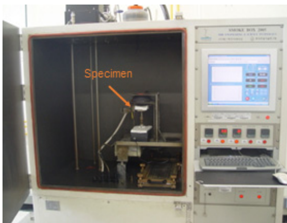
Fig. 4. Smoke generation test setup
