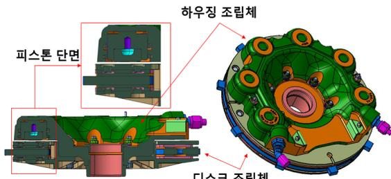
Fig. 5. Brake assembly of KT-1
