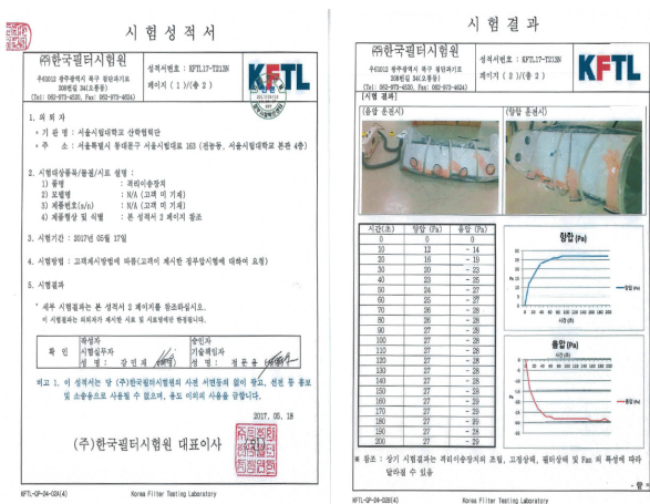
Figure 8. Result of HEPA filter leaks test.
