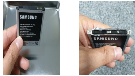
(a) Normal battery (b) Damaged battery
