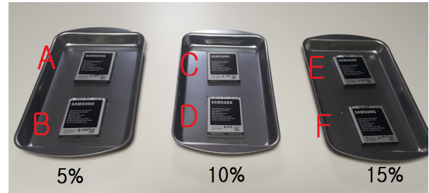
Figure 3. The battery submerged in salt water of different concentration (5 wt%, 10 wt%, 15 wt%).
