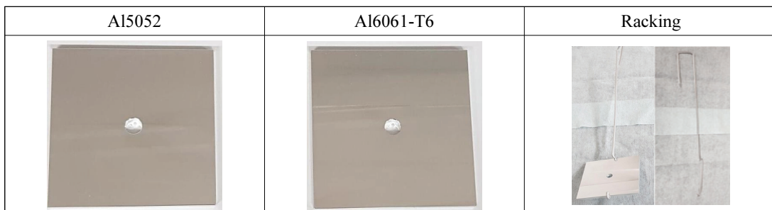
Fig. 1. Photographs of Al5052 and Al6061-T6 aluminum plate and racking used for anodizing.
