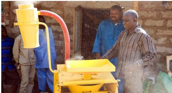
Fig. 4 Photograph of fonio husking machine in Senegal [15]
