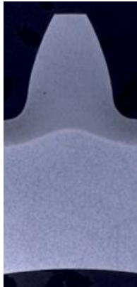
Fig. 6 Experimental results of single-frequency induction heating
