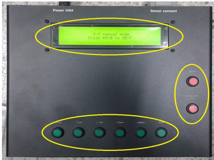
Fig. 5 Control box of programmable operation
