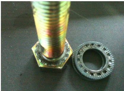
Fig. 9 Photograph of bolt and washers after 1,360 seconds vibration test
