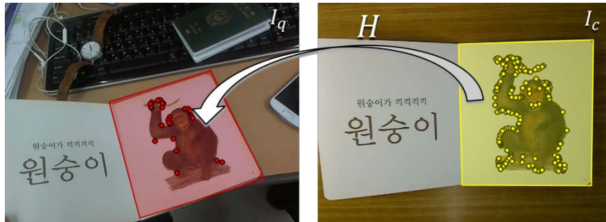
Fig. 9. An example of 2D transformation by using a homography.
