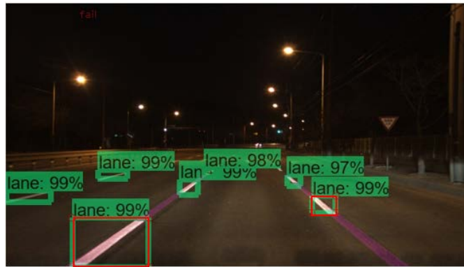
Fig. 11. Application of hybrid fusion algorithm and box selection for each lane
