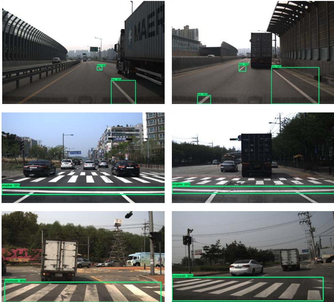
Fig. 13. Result of object detections on road
