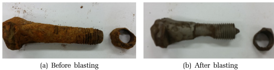
Fig. 4. Corrosion conditions of bolts and nuts before and after abrasive blasting.
