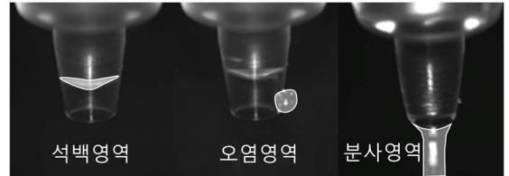
Fig. 3. Inspection region for detecting defect.
