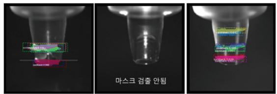
**Fig. 8.** Suck back region inferred by means of using Mask R-CNN without pre-processing.
