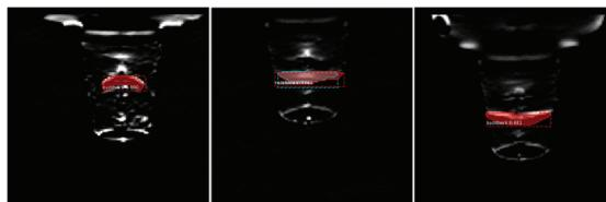
**Fig. 9.** Suck back region inferred by means of using Mask R-CNN with pre-processing.
