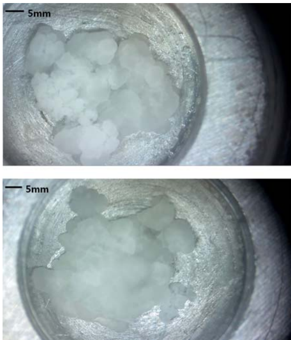
Fig. 11 Formed CP hydrate - MeOH 5 wt%, (Temperature : -10 °C)
