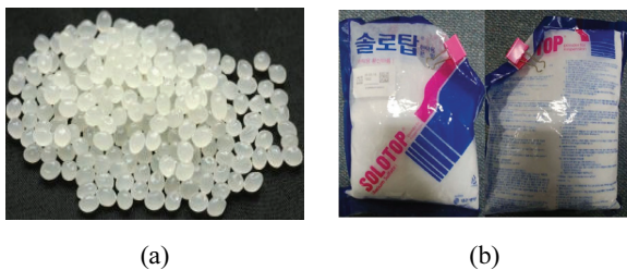
Fig. 1. Materials for fabrication of mixed radiation shield. (a) PLA pellets, (b) barium sulphate
