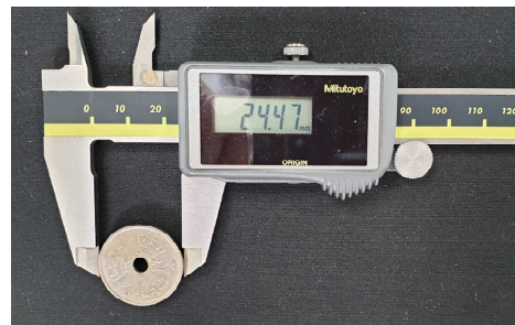
Fig. 7. A measured diameter of coin with a calipers
