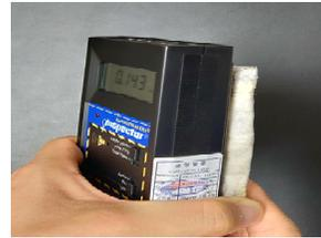
Fig. 4. Measurement of scatter using a dosimeter
