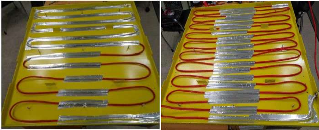
Figure 3. Comparison of heating cable installation (12 Line / 20 Line)
